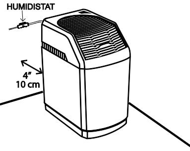
Do NOT position the unit directly in front of a hot air duct or radiator. Do NOT place on soft carpet.
