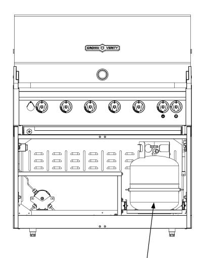
For LP applications that are not connected to a bulk supply, a pull-out propane tank drawer is factory installed along with a hose and regulator assembly to attach to a 20 lbs. tank (not supplied). A shelf is also installed to prevent the storage of a second propane tank per the residential standard for outdoor cooking appliances ANSI Z21.58-2018 and CSA 1.6-2018
