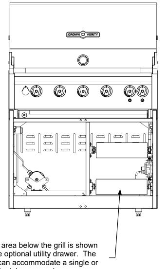
For LP applications that are not connected to a bulk supply, a pull-out propane tank drawer is factory installed along with a hose and regulator assembly to attach to a 20 lbs. tank (not supplied). A shelf is also installed to prevent the storage of a second propane tank per the residential standard for outdoor cooking appliances ANSI Z21.58-2018 and CSA 1.6-2018
