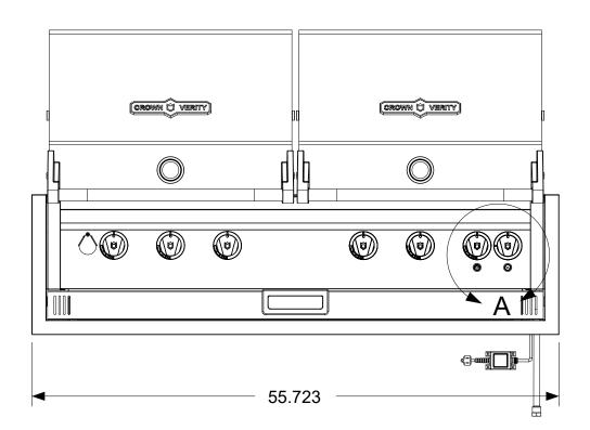
The dimensions shown are the actual physical dimensions of the grill. Additional clearances to cabinetry are dependent on the tolerances of the cut-out. The suggested cut-out dimensions are listed in the chart below but these dimensions can be reduced if the tolerances are controlled.
