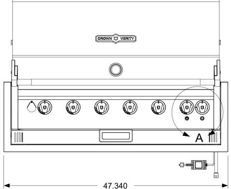
The dimensions shown are the actual physical dimensions of the grill. Additional clearances to cabinetry are dependent on the tolerances of the cut-out. The suggested cut-out dimensions are listed in the chart below but these dimensions can be reduced if the tolerances are controlled.
