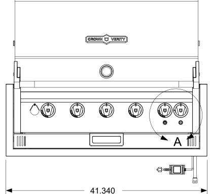
The dimensions shown are the actual physical dimensions of the grill. Additional clearances to cabinetry are dependent on the tolerances of the cut-out. The suggested cut-out dimensions are listed in the chart below but these dimensions can be reduced if the tolerances are controlled.
