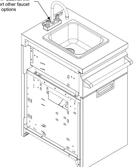
Storage area below the sink with optonal garbage drawer shown. If connecting directly to pressurized water and a waste water drain, optional drawer configurations are available at the time of ordering or can be installed at a later date. If purchased with the water heater option or the fresh and greywater tank options, drawer options are not available.
