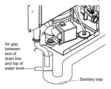
Figure 16: Example of an open drain.
