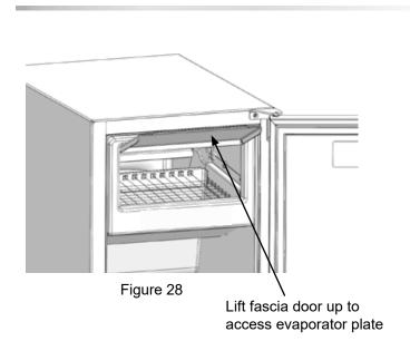
Refer to your cleaning solution instructions to determine the proper amount of cleaning solution to add based on 2 quarts (1.9 liters) of water. Lift fascia door up to access evaporator plate (See Figure 29). Pour the cleaning solution slowly on the evaporator plate so it flows down into the fresh water reservoir. (See Figure 30).
