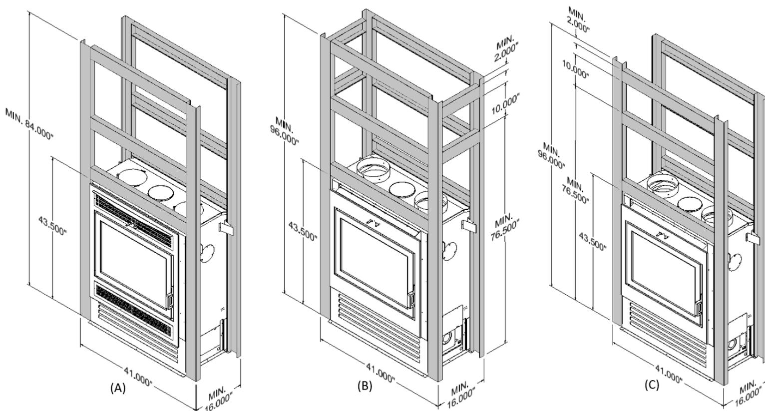
Figure 3-9: Astra Duo 38 Framing Design for (A) Traditional Surround Configuration, (B) Contemporary Surround with Side Wall 8" Gravity Ducts, and (C) Contemporary Surround Configuration with Front or Back Wall 8" Gravity Ducts
