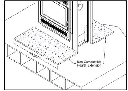
Figure 3-11: Astra Duo Hearth Extension Isometric View
