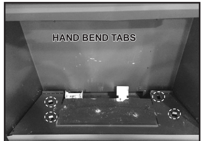
Figure 3. Hand Bend Tab Locations - QUARTZ36 Shown
