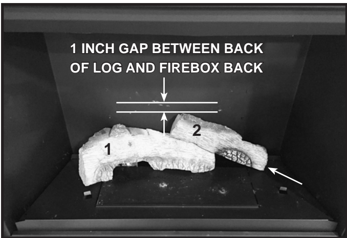
Figure 5. Install Right Rear Base Log
