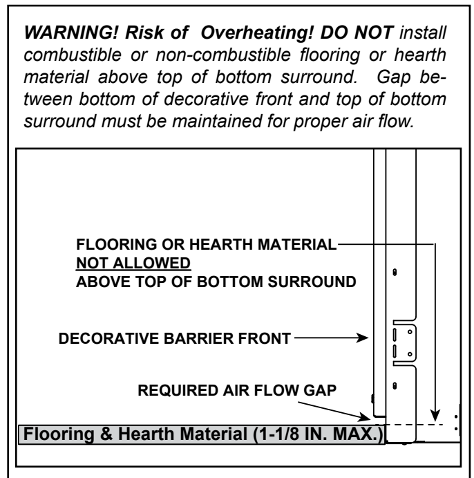
Figure 10.3 Required Air Flow Gap
