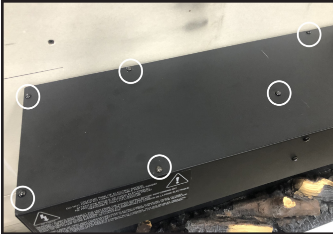
Figure 3 Appliance top panel removal showing left side screws (6 shown, 12 total)
