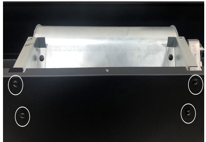
Figure 5 Heater assembly, screw removal location
