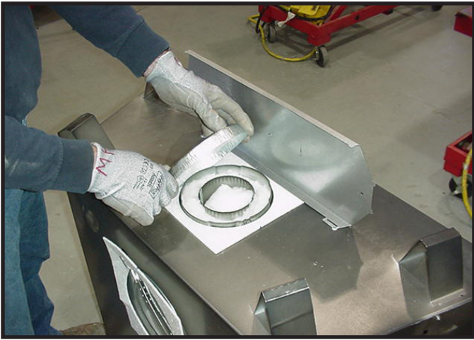
Figure 6.8 Remove the seal cap.
