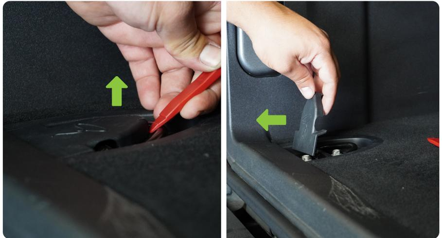
**STEP 5** | Use a 10mm socket to remove the hardware securing the factory tie-downs to the vehicle.
