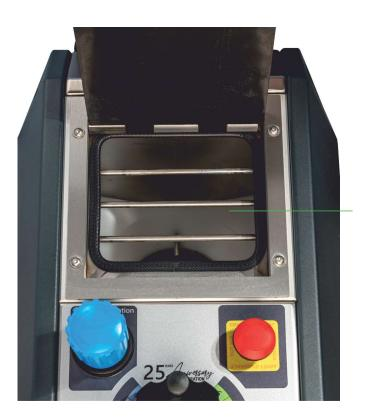
The moving parts of the machine are protected by a non-removable barrier located in the hopper neck.
