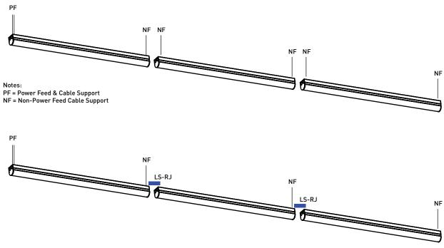
Notes: PF = Power Feed & Cable Support NF = Non-Power Feed Cable Support LS-RJ = Top Housing Aligner Accessory for Continuous Rows
