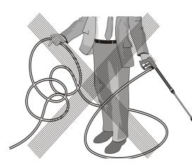
Never pull the high pressure hose if it has formed kinks or "nooses"! Never pull the hose over sharp edges!
