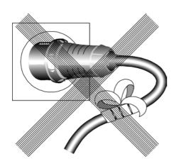
Do not damage the power cable or repair it incorrectly! (Replace defective or damaged cables immediately! Never work with a defective appliance!)
