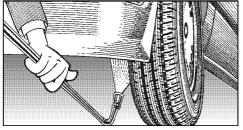
Underbody cleaning of cars, trailers and equipment: lance 90 cm with high pressure nozzle and ST 30 nipple M 22 x 1.5. The lance must be aimed when spraying. (See page 9)
