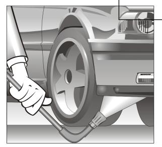
Always aim the underbody lance. Note when using an angled underbody lance, like for example lance no. 41.075 1, that there is a certain amount of torque in the recoil.
