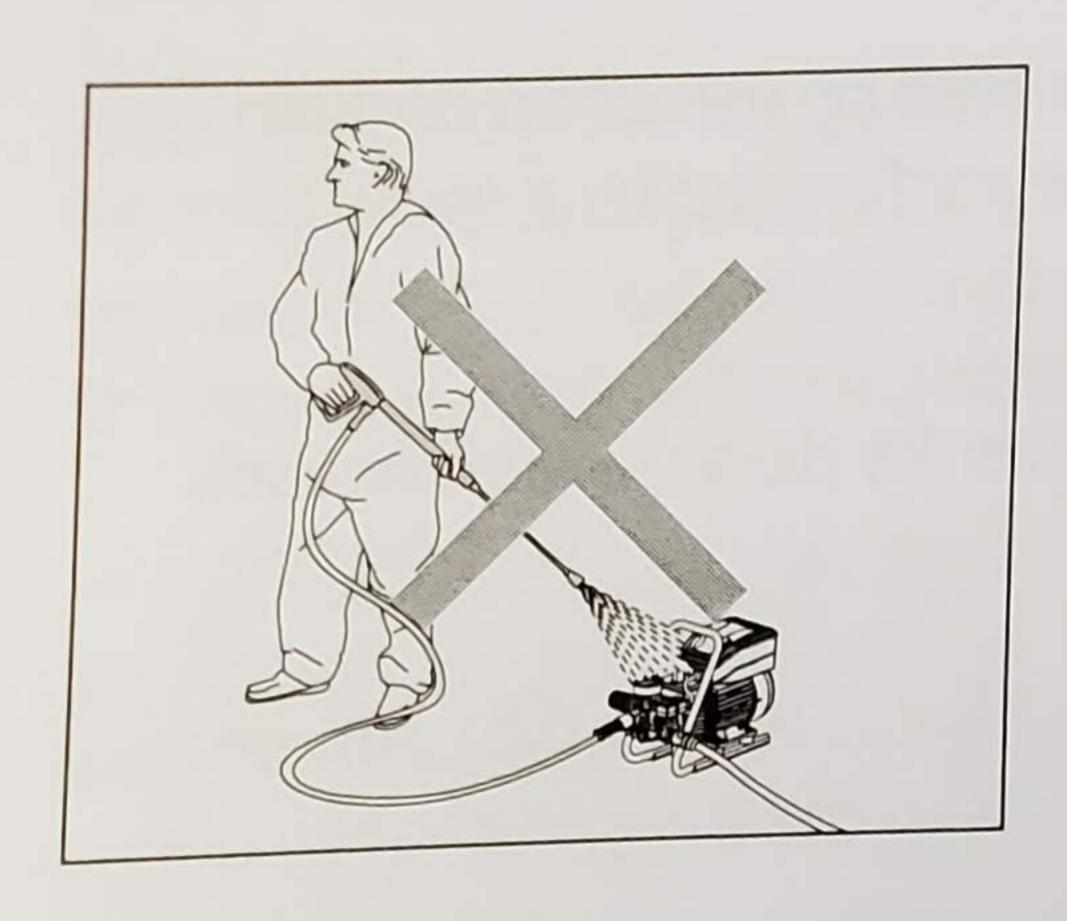
Never direct the high-pressure jet at the highpressure cleaner itself! The high-pressure cleaner may not be placed within reach of the highpressure jet spray mist!
