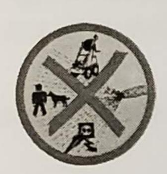
In case of improper use, the high-pressure jets can be very dangerous. Do not direct high-pressure jet at persons, animals or active electrical equipment or the high-pressure cleaner itself.
