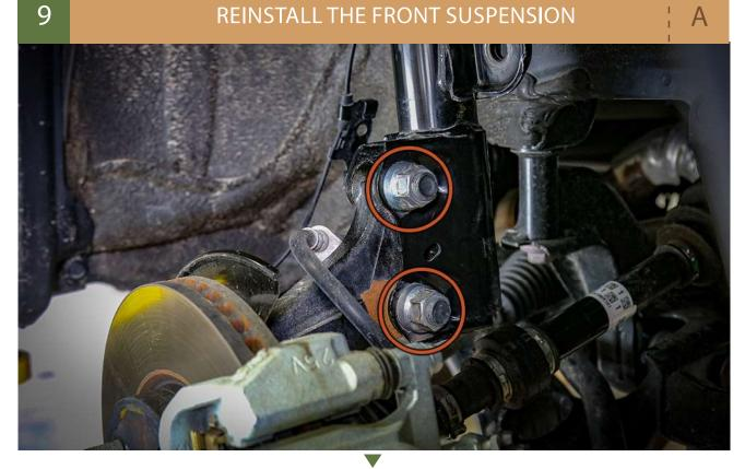
YOU MUST INSTALL THE BOTTOM BOLT FIRST.
