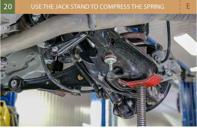
NOTE: Use the jack stand to compress the spring, it will lower the trailing arm, which will allow you to insert the spacer.
