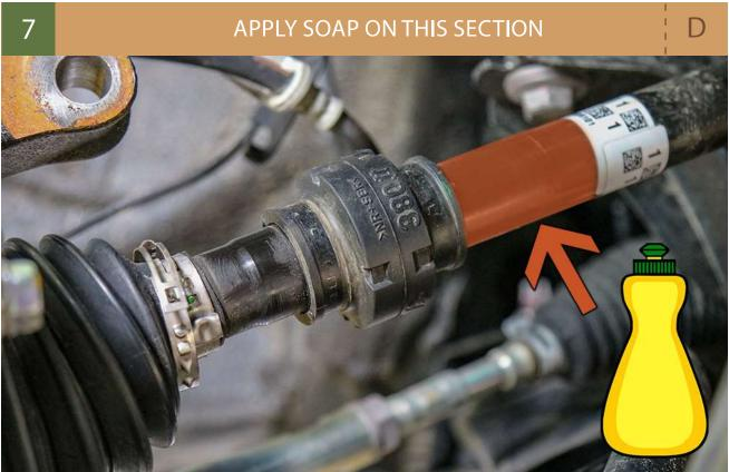
NOTE: The soap will allow you to slide the rubber damper on the axle. The soap will evaporate.
