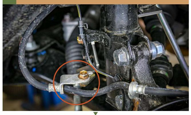
NOTE: You need to disconnect the ABS sensor, and reconnect it so that the wire is between the brake line and the shock.
