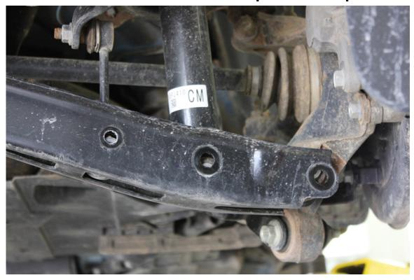
Note: You must remove the carpet and plastic covers in the trunk to gain access to the suspension bolts.
