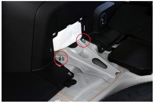
10. Unbolt the bottom and the top of the rear suspension
