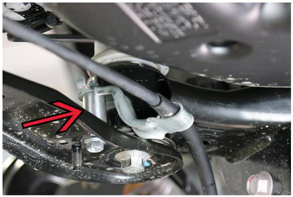
**20.** Use the Z-shaped bracket to re-install the mud flaps
