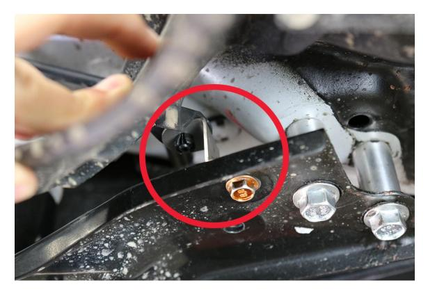
**21.** Reinstall the brake lines with the brackets
