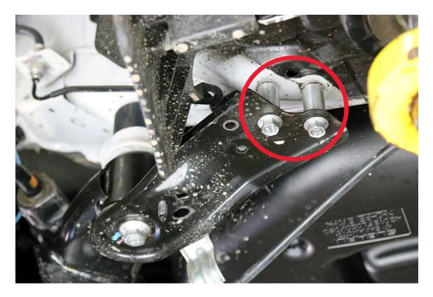
\*\*\* install the e-brake bracket in this way, using the spacer\*\*\*
