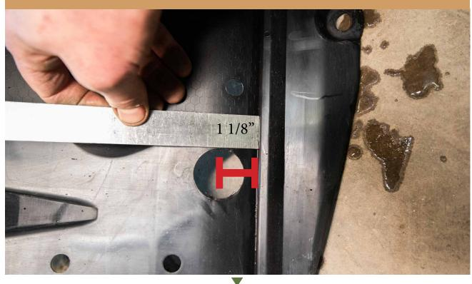
USING A HOLE SAW, DRILL OUT THE HOLES
