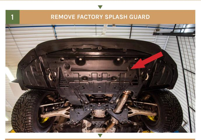
YOU NEED TO REMOVE THE SPLASH GUARD IN ORDER TO MAKE TWO HOLES IN IT TO BE ABLE TO MOUNT THE BUMPER GUARD TO THE RAD SUPPORT
