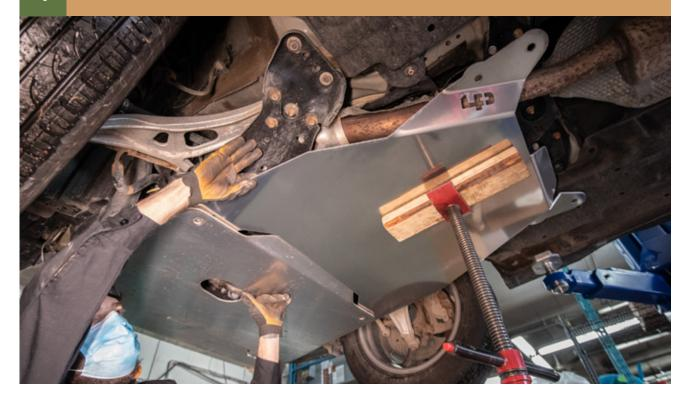
5 PLACE THE FRONT OF THE CVT SKID PLATE OVER THE REAR OF THE MAIN SKID PLATE.
