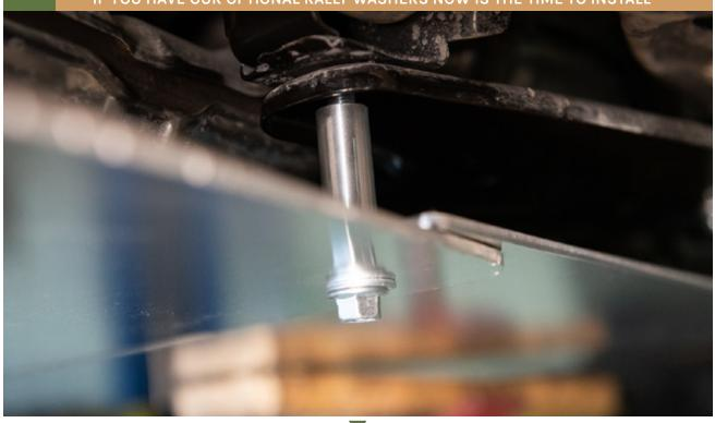
BOLT UP REAR OF THE CVT SKID PLATE.
