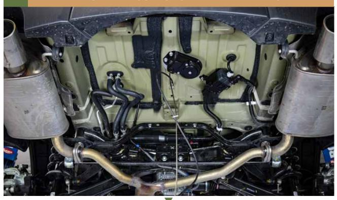
UNSCREW THE 4 BOLTS OF THE SUBFRAME BRACE
