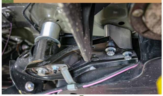
31 INSTALL THE SPACERS OF THE SUBFRAME BRACE (BAG #4B)
