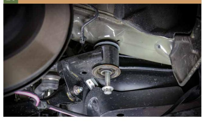
**NOTE :** Temporarily install the front bolts, keep the subframe properly aligned. This will help you for the nexts steps of the installation.
