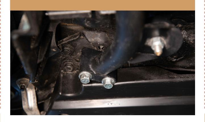
6B FOR LIFTED VEHICLES THE ROCK SLIDER GOES INBETWEEN THE SUB FRAME SUPPORT AND THE UNIBODY. USE THE BOLTS FROM THE LIFT KIT TO INSTALL
