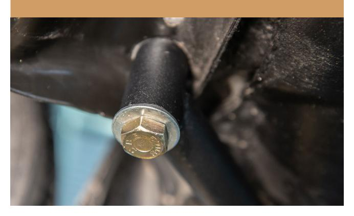
FOR NON LIFTED VEHICLES THE REAR OF THE ROCK SLIDER GOES UNDER THE SUBFRAME SUPPORT. USE THE BOLTS PROVIDED IN THE ROCK SLIDER KIT TO INSTALL
