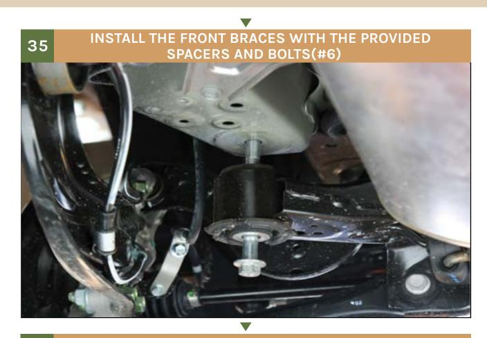
**35** DO NOT COMPLETELY TIGHTEN THE BOLTS AT THIS STEP
