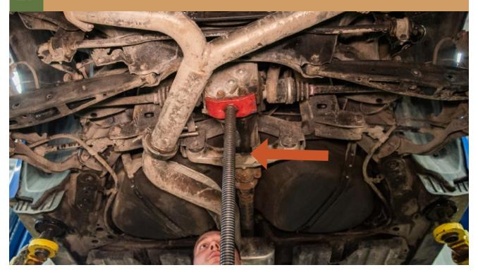
REMOVE THE FRONT BOLT OF THE REAR SUB FRAME WITH ITS SUPPORT BRACKET
