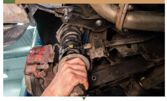
RE INSTALL KNUCKLE, STRUT AND SWAY BAR BOLTS
