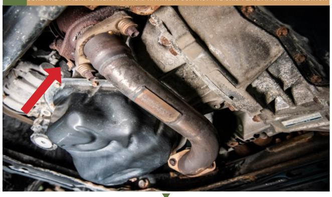
THREAD IN THE SKID PLATE SPACERS. THE SPACERS WILL BE LONGER IF YOU ARE INSTALLING WITH A STOCK FRONT PIPE
