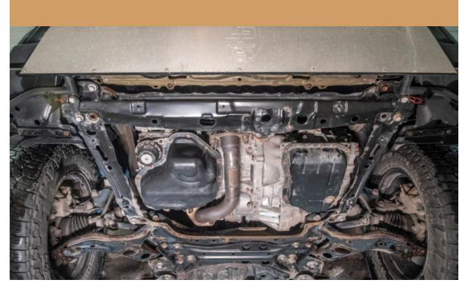
2 IF YOU HAVE A LACHUTE PERFORMANCE FRONT PIPE, NOW IS THE TIME TO INSTALL IT. MAKE SURE THE FITMENT IS TIGHT TO AVOID HAVING IT CONTACT THE SKID PLATE AFTER INSTALLATION
