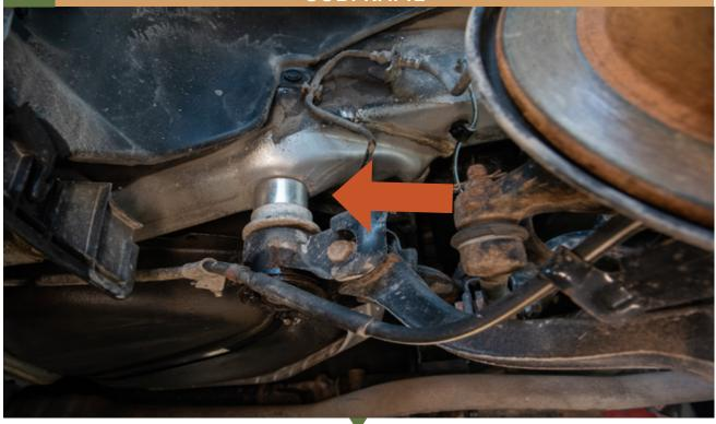
RE INSTALL SUPPLIED SUBFRAME BOLT WITH THE SUBFRAME SUPPORT BRACKET
