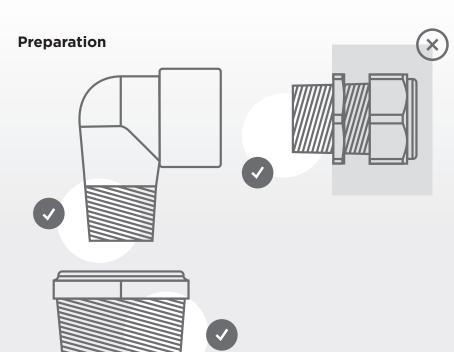
**DO NOT** apply Teflon tape on the <u>front nut</u> of the cord grip.
