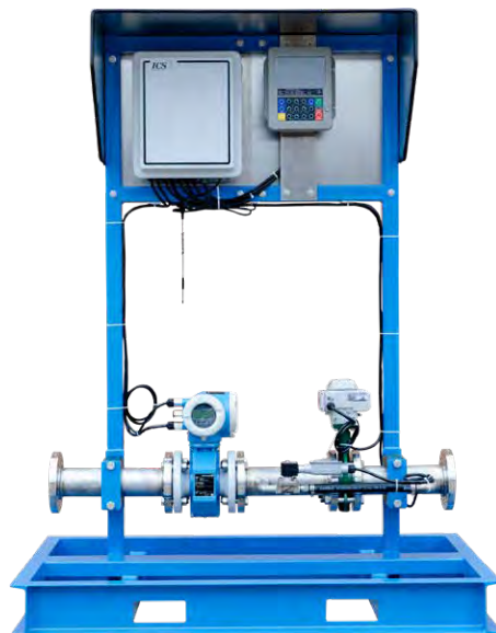
Example loadout skid using the TCS 3000 as the unattended loadout flow computer, along with an NTEP approved MAG meter and high flow/low flow valves.
