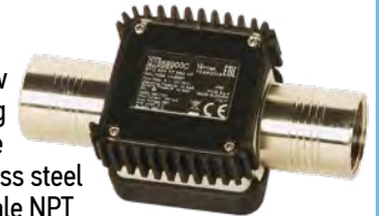
P/N 560038 In Line Electronic DEF Turbine Meter, 1" NPT inlet/outlet with flow range of 2 – 35 GPM, +/- 1% accuracy, 50 PSI operating pressure. Uses 2 ea. AA batteries, units of measure can be easily changed from pints to quarts, liters or gallons. Polypropylene construction with an operating temperature of 0° F – 130° F. For use with DEF, Anti-Freeze, De-Icing fluid and Non-Potable water.
