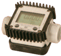
P/N 100388 DEF turbine pulse meter has a flow range of 1.5 – 26 GPM and working pressure up to 145 PSI. Fittings are 1" male BSP and two each stainless steel adapters, 1" female BSP x 1" female NPT are included.
