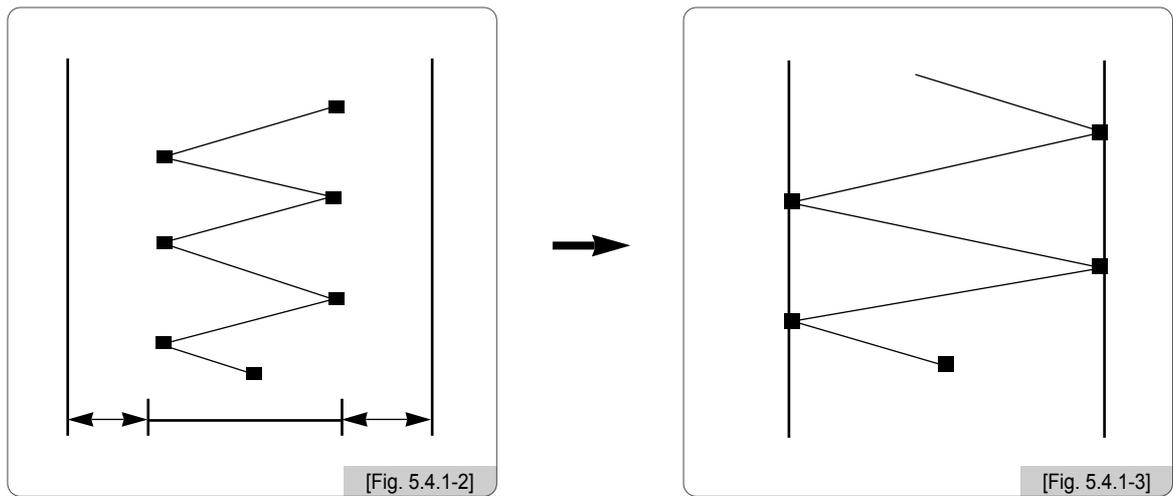
This function determines the satin stitch length in the X-axis direction. The value can be increased by the unit of 0.1mm.
