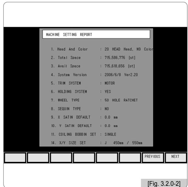
Use **F1** (left arrow), **F2** (right arrow) to move to a desired item and press **F7** SELECT . Then the screen like 'Fig. 3.2.1 Embroidery Machine Specifications Setting' appears where the setting of each item is possible. When the setting is completed for all items, press **F7** NEXT . <Fig. 3.2.0-2> appears to check the set specifications.
