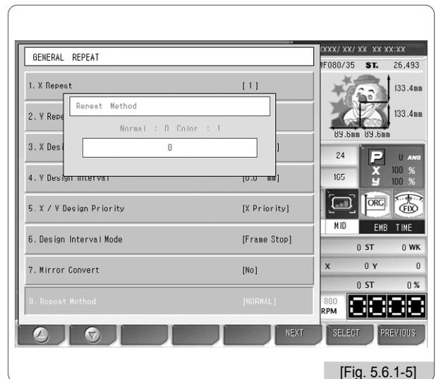
© If the repeat type is COLOR(1), “7. Mirror Convert” cannot be used. If the repeat type is NORMAL(0), the function can be used.
