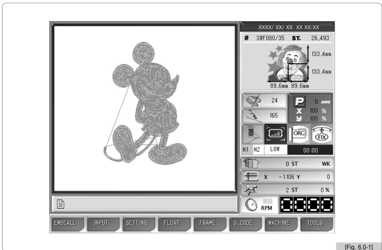
In this section, the explanation will focus on the different part of the menu compared with the menu before embroidery begins, such as “EMBCall”, “Setting”, “Float”, “Frame”, and “S\_Code”.
