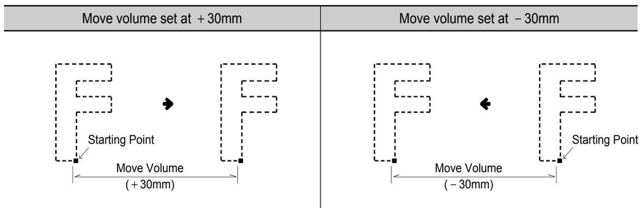
④ Y Design Interval : It sets the distances between the starting points of the repeated design along the Y axis.
