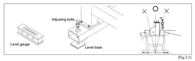
2) The machine must be horizontally balanced on all four sides - front, rear, right, and left.
