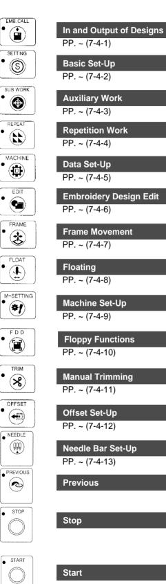
reads in or outputs designs basic set-up (scale up/down, rotation, etc.) measures length, checks paths, etc. repetition work sets up embroidery related data edits embroidery designs (STOP mode) or changes speed (OPERATION mode) moves the frame non-stitching functions machine set-up copying, deletion, formatting, etc. manual trimming set-up offset set-up the needle bar
