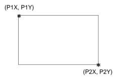
It produces an error message when the embroidery material goes over the frame limit set. To have the error message function, select "DATA SET-UP"  $\rightarrow$  "EMB FUNCTION"  $\rightarrow$  "15] FRAME LIMIT" and set "YES." This function is not available on SWF/ $\Box$ -W1201 and SWF/ $\Box$ -1204.
