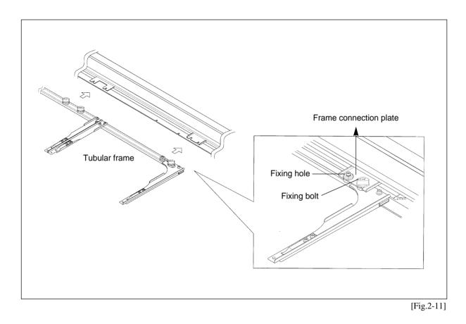
2) Insert the frame into the tubular frame. Use the screws to adjust the space.
