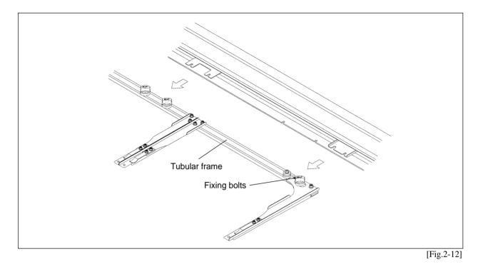
1) Unfasten screws on the tubular frame 2/3 and remove the frame.
