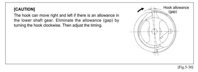
2 Adjusting Gap between Needle and Hook Point
