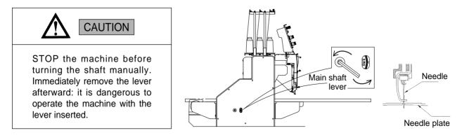
② When inserting the needle, make sure that the groove of the needle is facing front. Shaft of the needle should be inserted completely into the needle bar.
