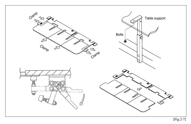
2) Adjust the table support at an appropriate height and fasten the bolts.
