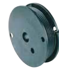
DeLaval ground cable Connect earthing rods and gateways above or below ground. The cable is double insulated and features a galvanized steel wire conductor. Voltage strength approx. 20 000 V. The cable is available in three different lengths: 10, 25 and 100 m. Ø 1.6 mm, 10m. Art. no. 86675501 Ø 1.6 mm, 25m. Art. no. 98767235 Ø 2.5 mm, 100 m. Art. no. 88859601
