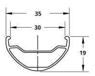
Join: Pin Spoke: 32H Finish: Sandblast Anodised Weight: 525g(29")
