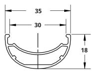
Join: Welded Spoke: 28H Finish: Sandblast Anodised
