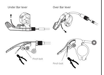
Step 6. Attach the remote lever to the handlebar, position this close enough to the handlebar grip that the riders thumb can press the lever. Once the lever is attached securely the cable tension must be adjusted. This can be done by using barrel adjuster. The cable should have 1-2mm of play and should not be under tension. If tension is too high the dropper post may actuate unintentionally.
