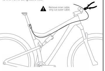
Step 2. Push on the plastic cable ends on to the outer cable. The inner cable must be fed into the outer cable from the dropper post side leaving around 30mm of exposed cable before the cable end stopper.
