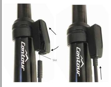
Step 5 . Loosen the pinch bolt on the lever. Insert the inner cable through the lever and push the outer cable end in to the tensioner. Tighten down the pinch bolt to clamp the cable. Cut the inner cable. Install and crimp the cable end ferule onto the end of the inner cable.
