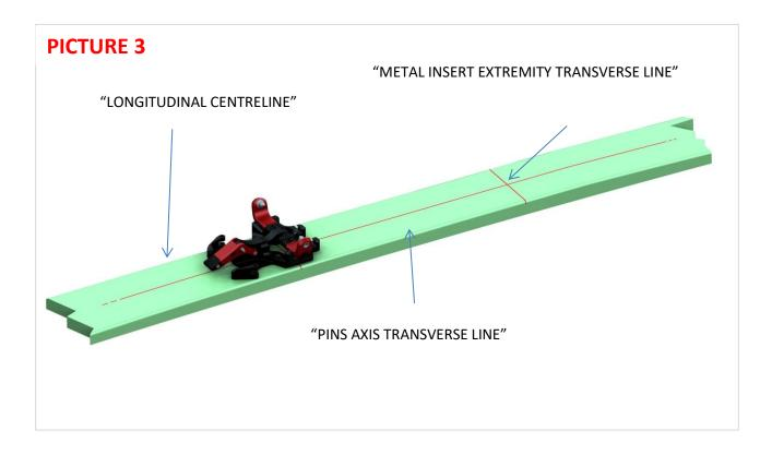
10) Hook the boot to the toe part , place the sole on the skis and draw the rear "METAL INSERT EXTREMITY TRANSVERSE LINE" of the boot ( PICTURE 4 ).
