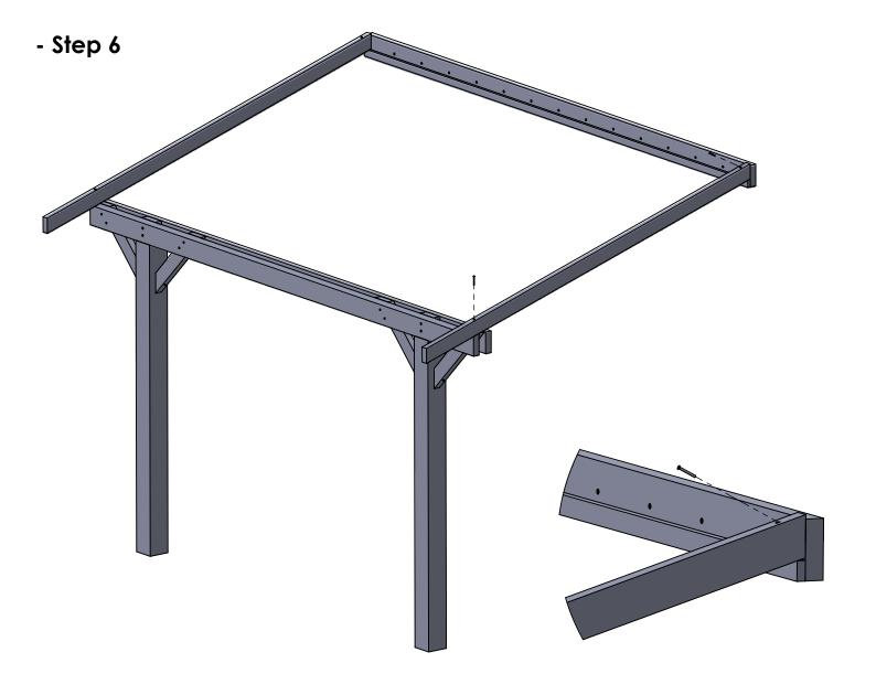
Begin by positioning the two outermost rafters (Part E). These should sit on top of the ring beam and rest securely on the support batten. Align each rafter so it is flush with the ends of both the ring beam and the wall plate. To fix in place, drive one 6.7mm x 125mm screw vertically down into the ring beam. Then, angle a 5.0mm x 100mm screw through the top of the rafter into the wall plate to secure it firmly.
