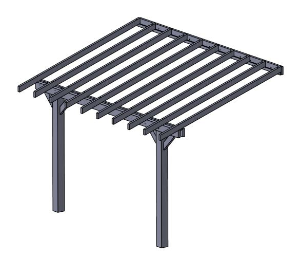
Now, repeat the process from Step 6 to install the remaining rafters (Part E). Position them evenly along the length of the lean-to, using the same method to secure them—one screw into the ring beam and one angled screw into the wall plate. Rafter spacing should be indicated by pre-marked positions on the ring beam.
