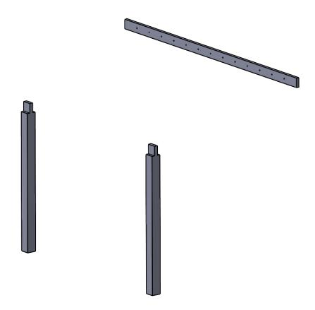
With the wall plate securely in place, the next step is to set the vertical support posts. A lean-to pergola typically requires 2 or 3 posts arranged in a straight line, set parallel and square to the wall plate, rather than in a square layout like a freestanding pergola.
