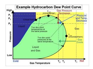
Figure 1 Example Hydrocarbon Dew Point Curve
