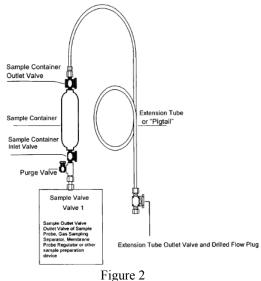
Purging, Fill and Empty and Purging Controlled Rate Methods Example Sample Setup
