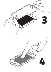
Align glass protector with your device by holding the easy-apply tabs. Press & hold down the center of glass with your finger, then peel off the easy-apply tabs. (Use microfiber cloth to work out any air bubbles that may have formed, and allow 1–2 days for smaller bubbles to fully disappear.)
