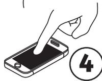
Tip: If any dust particles remain under glass, carefully lift glass up, starting at a corner, and use dust removing tabs to get rid of dust. Set protector back onto screen.
