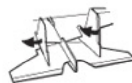
a Correction: Bend the rudder to left.
