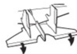
c Correction: Bend the elevator slightly downward.
