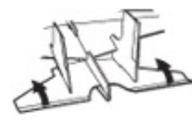
d Correction: Bend the elevator slightly upward.
