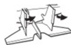
b Correction: Bend the rudder to right.
