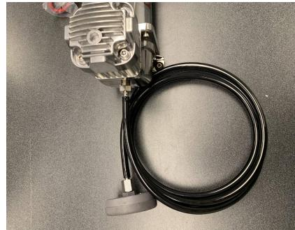
Route the air filter up to a high and dry location where it will not get wet or exposed to the elements. The compressor itself is fully sealed but if your filter gets wet, the compressor can pull water into itself and this will lead to problems later on down the road. Your compressor will last much longer if the filter is relocated to a high and dry location. Be careful not to kink the air line while routing the filter around.
