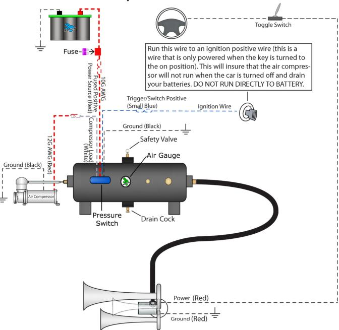
Warning: To ensure the life of your system, reading and following these instructions are recommened. Make sure to change filters and to drain the moisture from the tank on a regular basis. Most factory horns are positively activated. If your horn system is negatively activated, then you will need to wire one of the leads from the valve to a direct 12v power source. Then wire the other lead to the negatively charged horn wire.
