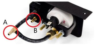
will connect out to the air bags in the rear of the vehicle. Barb fitting 'B' will connect to the ¼" line coming out of your air tank. Once plumbed, move the valve up to test the flow of air through the system. Air should flow from the tank to the bags.
