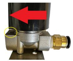
Wrap a small amount of Teflon tape around the ¼" NPT x 3/8" Elbow fittings. Plumb this fitting into the bottom-most port of your air tank. Gravity will pull water into the fitting from the tank. The fitting must be on the bottom of the tanks for this to work
