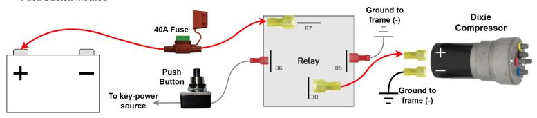
Start by cutting the fuse holder in half to make two ends. Connect one end to the battery. Use a butt connector on the opposite end to run 10-gauge wire to pin 87 on the relay. You will also use a section of 18-gauge wire from the end of the fuse holder to the push button. Use the red 10-gauge (larger) wire from pin 30 to the compressor, as well as for the compressor ground. Use 18-gauge (smaller) wire from the push button to pin 86, and from pin 85 to the desired ground point.
