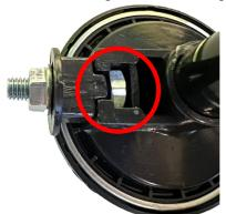
the nut on the bolt and tighten it down. Don't overtighten it or the plastic will break. You will repeat this process for all five horn bells.
