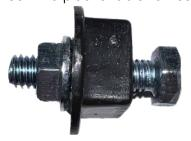
Locate one of the horn bells. The head of the bolt will slide into the base of the horn as shown below. Make sure the alignment tab for the plastic mount is lined up with the slot on the horn as circled below. At this point, the horn is ready to be mounted. Once your mounting hole is drilled, remove the nut from the bolt and insert the bolt through the mounting hole. Re-thread
