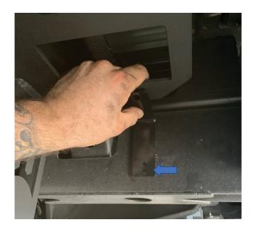
• Install the L bracket on to the horn mount using the provided stainless hardware. Once installed, drill a 5/16" hole into the hitch.
