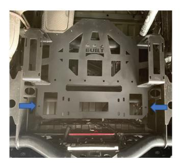
• Put the mount on unloaded, snug the hitch nuts you removed. Install L-brackets to thes holes circled in the picture above.
